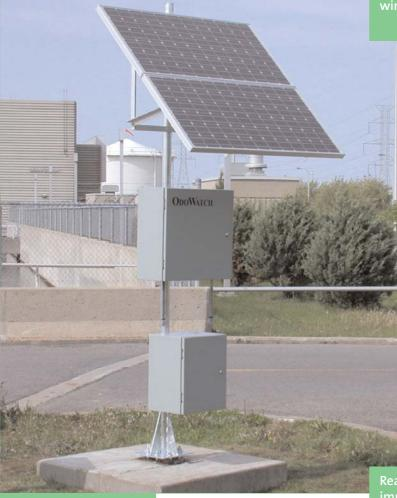
OdoWatch™ is the world's first electronic nose network for 24/7 wireless odour monitoring.
