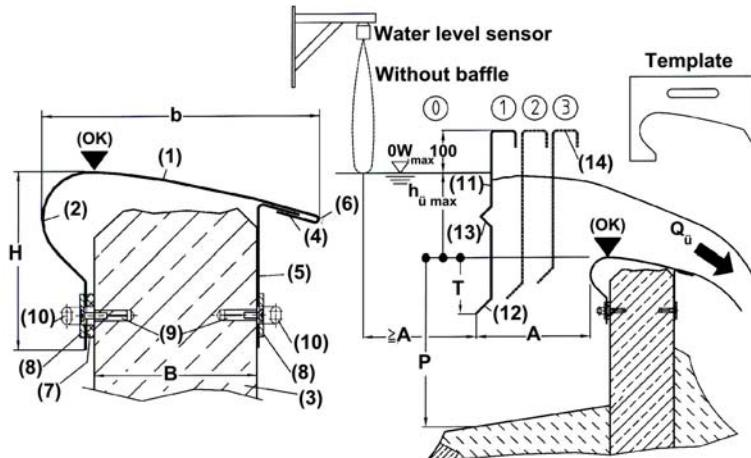
**Figure 1: Hydrovex® FluidWing Installation**
