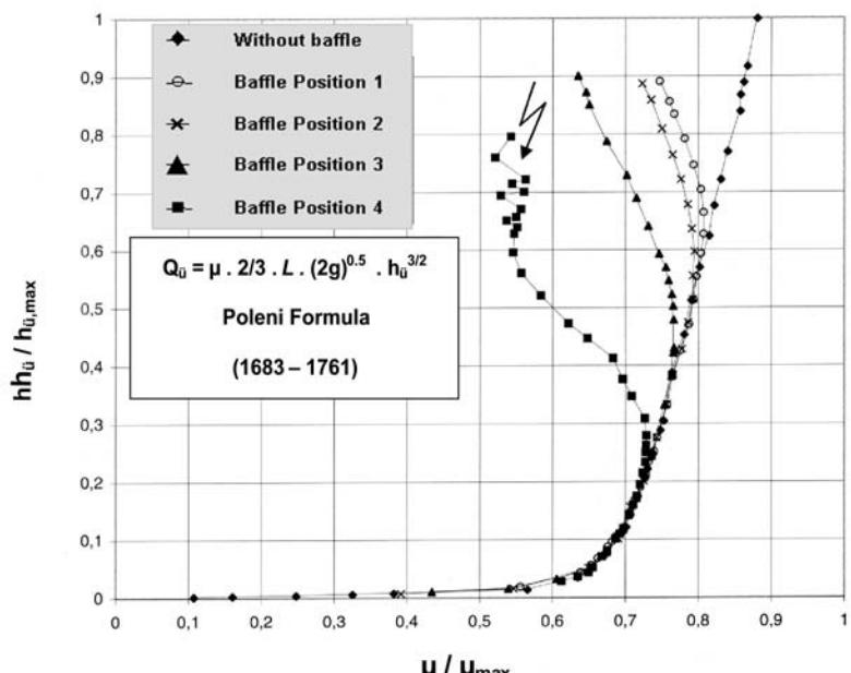
**Figure 3:** *Measured discharge*
