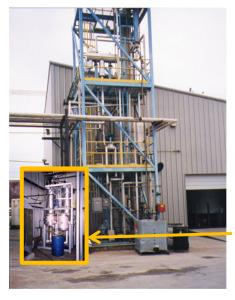
Much more compact and robust than Steam stripper. Suitable for indoor placement
